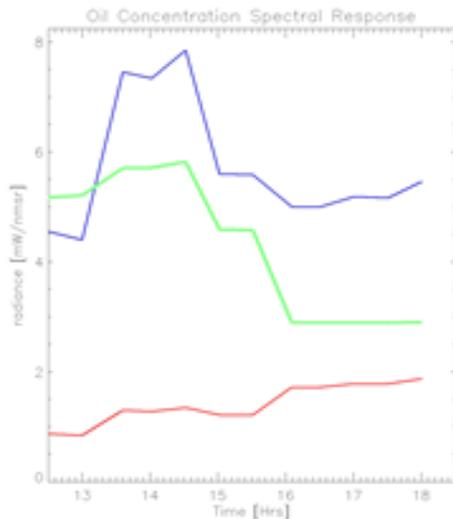
Figure 3. Time series of 615 nm (blue) and 710 nm (red) wavelength. With 25% oil added at 13:15, 50% at 14:30 and 100% at 16:40 UTC. Green is ratio 615/710 radiances. Absolute value depends on light source.
