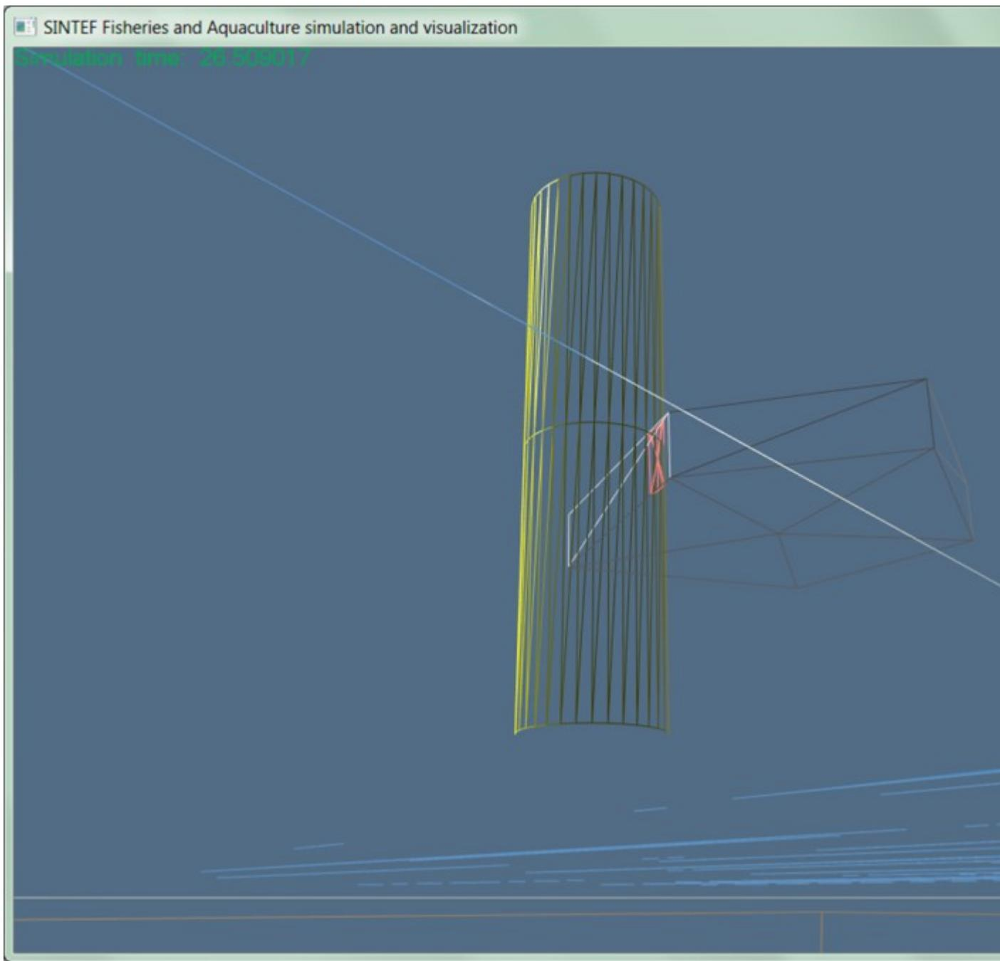
Figure 2. A screenshot from the preliminary simulation of wave-driven impact of an ice floe on a vertical circular cylinder (by FhSim)
