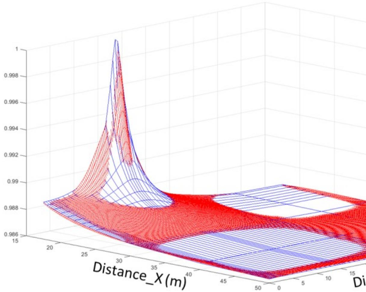
Figure 4. An example of the calculated (by WAMIT) and fitted add-mass coefficient
