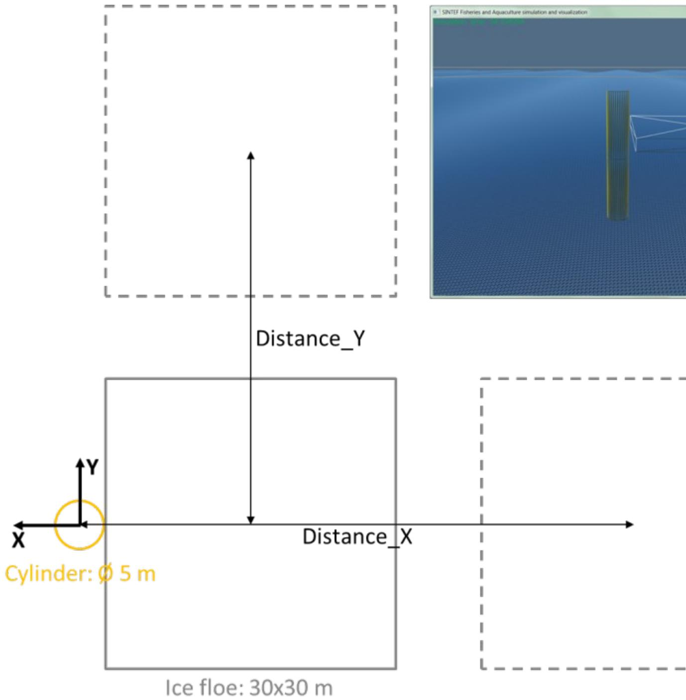
Figure 3. Illustration of a square ice floe approaching a circular cylinder (driven by wave)
