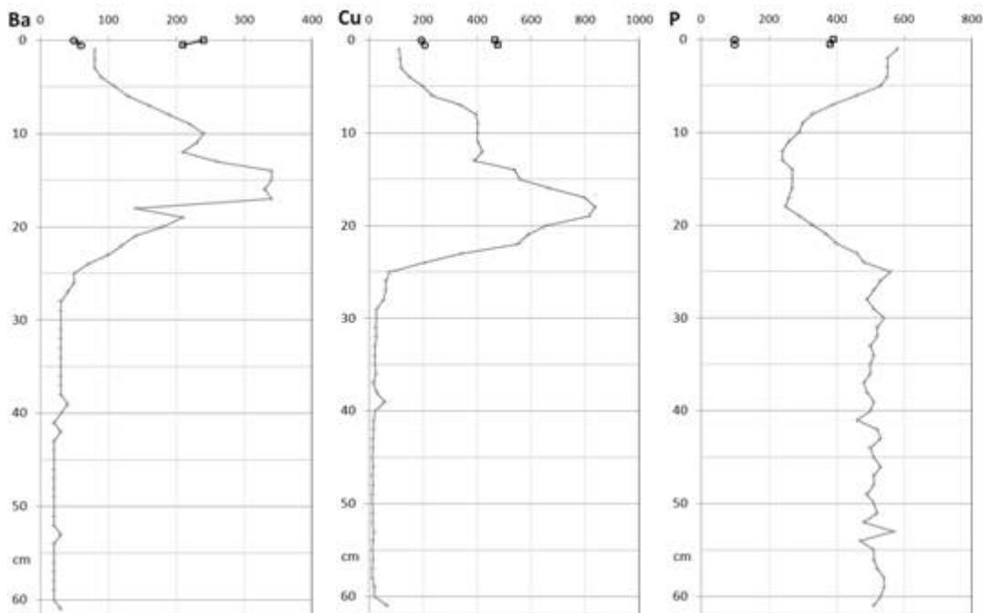
**Figure 1: Examples of elements within the longer core, which defines the chemical signature. The tailings material is present in a horizon at 5-25 cm depth. The markers at the top of the diagram show the analytical results for the fresh tailings from Ulveryggen (circles) and Nussir (squares). All samples are extracted by Aqua Regia.**
