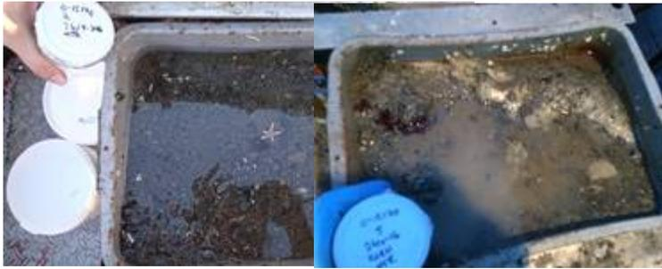
**Figure 3.** Boxes that had been placed on the seafloor in Repparfjorden from June 2015 – September 2016. Left: Control (no tailings). Right: 14.5 mm tailings.
