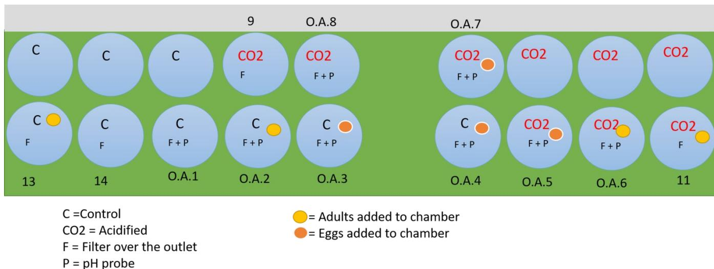
Fig. 1: Experimental set up of OA tanks for mortality estimates of *A. longiremis*.
